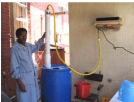
Halibet hospital technician holds AQUACHLOR generator (white cylinder) which converts brine in blue tub into sodium hypochlorite. Photo by Waverly Rennie.
